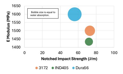
Origin has a robust portfolio of tough materials featuring different colors, performance profiles, and cost points. The three materials shown above are good choices for parts and applications in high impact environments (manufacturing jigs) or frequently opened and closed (latches).
